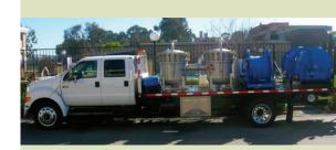
To flush the system, New Jersey American Water will be using a new technology. The water mains will be flushed by connecting fire hydrants to a self-sufficient trailer outfitted with filter vessels.
